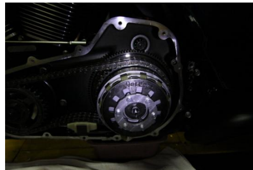
New clutch spring and Clutch Wiz spring retainer installed
