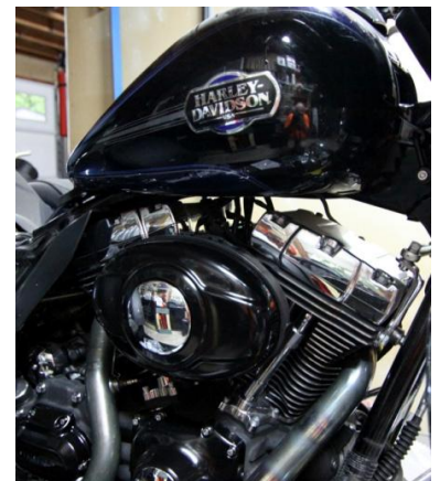
Fuel tank after 2 inch tank lift
