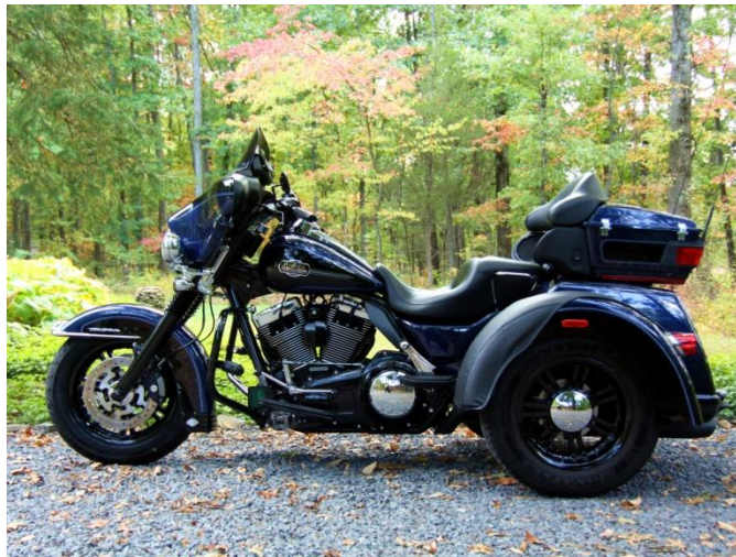
Trike with powder coated wheels and powder coated front end
