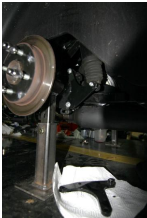
Replacing shock mount brackets with after-market brackets with 1.25 inch lift
