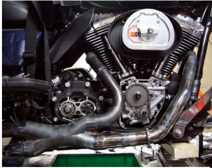
Air cleaner-trans covers and exhaust shields off to be powder coated
