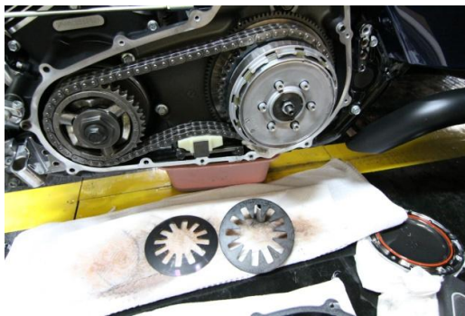
Stock clutch spring on left Evolution clutch spring on right
